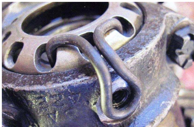
New homemade safety clip installed
