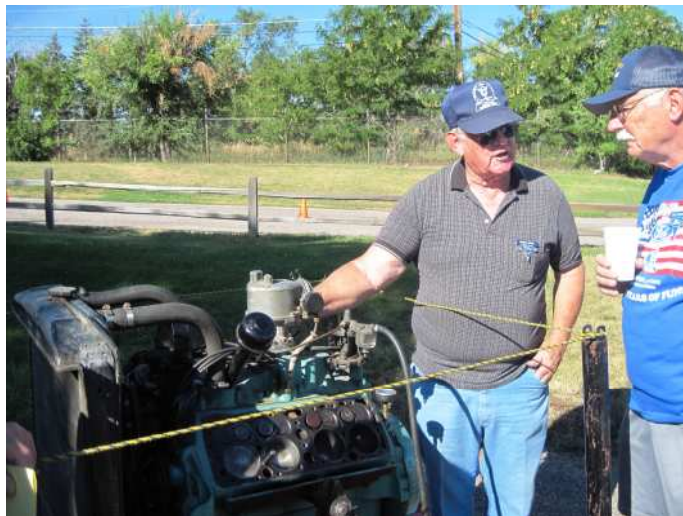
Bernie Sawin explaining the 4 cylinder operation of his V8 flathead at All Ford Day. Notice the missing head which provides for viewing of the flathead piston and valve operation. Photo by Ed Rockwell
